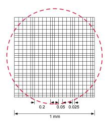
The depth of the Neubauer chamber is 0.1 mm.
